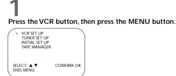
Press the PLAY  $\blacktriangle$  or STOP  $\blacktriangledown$  button to select VCR SET UP, then press the OK/STATUS button.
